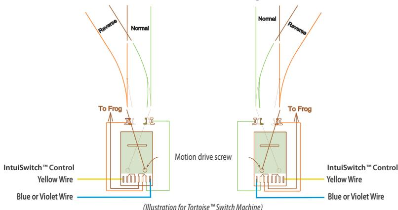
Route follows turnout to side of motion drive screw. The wiring for an insulated-frog turnout is shown. Either set of Tortoise™ switch contacts may be used. Connect the three conductors used for the frog connection (for example, - green, brown, and orange) as shown in the illustration.
