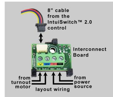
The controller can be powered by 12-24 Vdc (15 Vdc is recommended), 10-16 Vac, or DCC track power. Because each turnout's stall motor draws power (18 mA with the controller), connecting many controllers to track power reduces the power available to the trains. A separate dedicated source is recommended. Connect the power to the black (-) and the red (+) screw terminals on the breakout board, observing polarity if using a DC power source.
