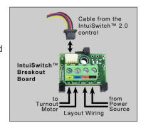
The controller can be powered by 12-24 Vdc (15 Vdc is recommended), 10-16 Vac, or DCC track power. Because each turnout's stall motor draws power (18 mA with the controller), connecting many controllers to track power reduces the power available to the trains. A separate dedicated source is recommended. Connect the power to the black (-) and the red (+) screw terminals on the breakout board, observing polarity if using a DC power source.
