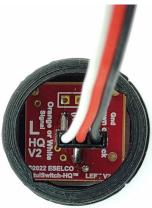
Orient the cable so the Orange or White wire goes to the pin labeled "Orange or White", and the Brown or Black wire goes to the pin labeled "Brown or Black"
